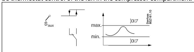
The thermostat can either use one of the sensors used by the regulation (Ss, Sd, Sc3) or an independent sensor (Saux1, Saux2, Saux3, Saux4).
