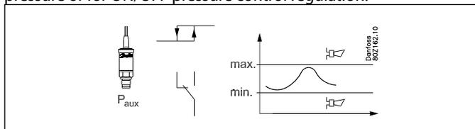
The pressure control can either use one of the sensors used by the control function (Po, Pc) or an independent sensor (Paux1, Paux2, Paux3).
