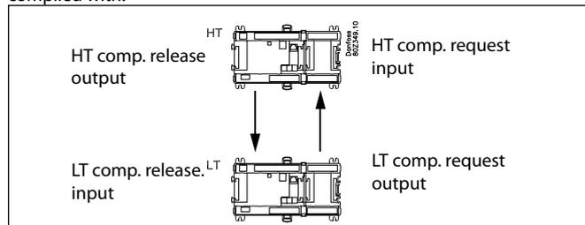
Here both a relay output and an On/off input are used on both controllers.
