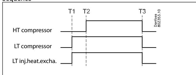
T1: The load on the low-pressure circuit requires compressor capacity.
