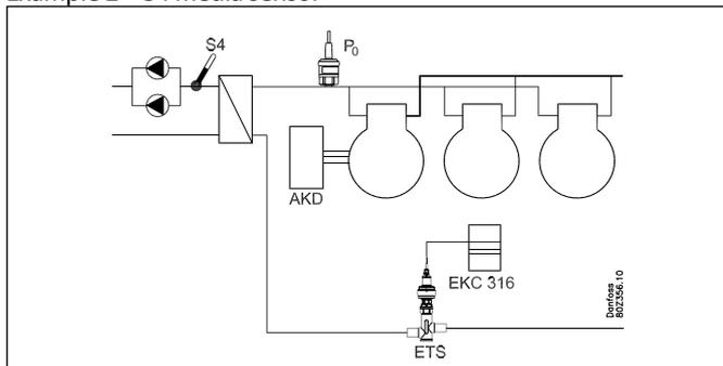
When the controlling sensor is selected as  $S_4$ ,  $P_0$  is used as a safety function for low suction pressure and will ensure disconnection of compressor capacity (frost protection).
