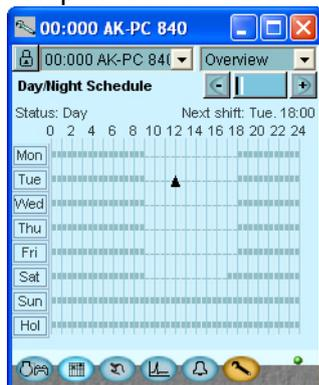
Before regulation is started we will set the schedule function for the night setback of the suction pressure. In other cases where the controller is installed in a network with one system unit, this setting may be made in the system unit which will then transmit a day/night signal to the controller.
