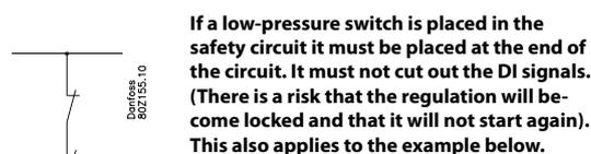
If an alarm is needed which also monitors the low-pressure thermostat, a "general alarm" can be defined (an alarm that does not affect the control). See the following section "General monitoring functions".
