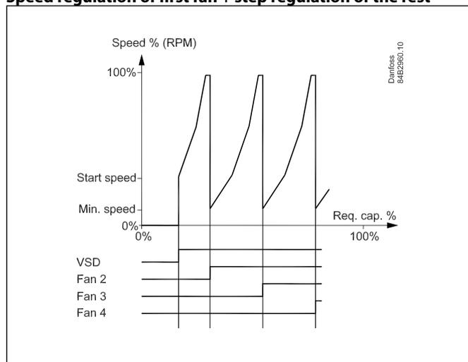
The controller starts the frequency converter and increases the speed of the first fan.
