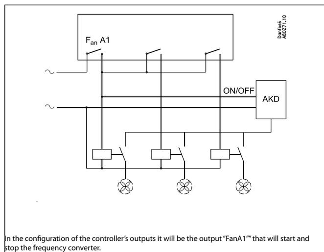
In the configuration of the controller's outputs it will be the output "FanA1" that will start and stop the frequency converter.
