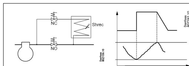
In both cases it applies that when the heat recovery function is de-activated, the reference for the condensing temperature will then decline slowly in accordance with the set rate in Kelvin/minute.
