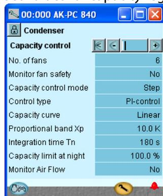
In our example the condenser pressure is controlled on the basis of the outdoor temperature (floating reference). The settings shown here in the display.
