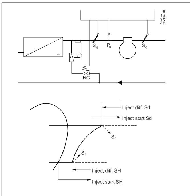
The high-pressure gas temperature can be kept down by means of liquid injection into the suction line.
