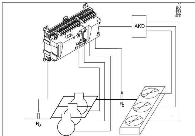
The controller's main function is to control compressors and condensers so that operation all the time takes place at the energy-optimum pressure conditions. Both suction pressure and condensing pressure are controlled by signals from pressure transmitters.
