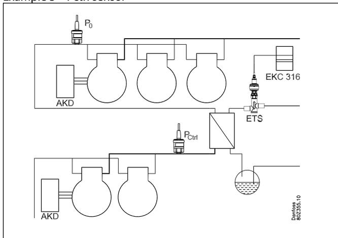
When  $P_{ctrl}$  is used as controlling sensor, a refrigerant type for this pressure transmitter must be set, e.g.  $CO_2$ .
