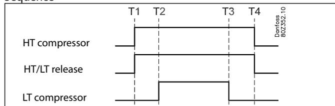
T1: First high-pressure compressor starts and the release signal is activated
