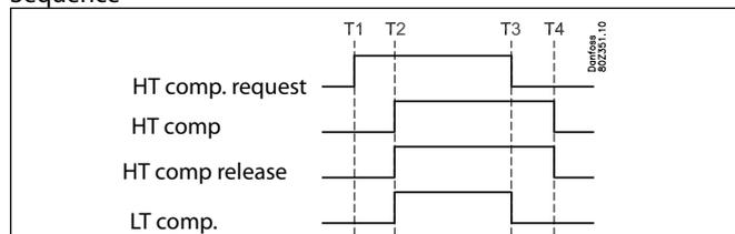
T1: The load on the low-pressure circuit requires that compressor
