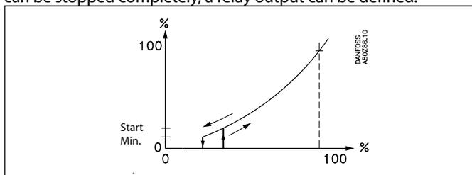
The controller starts the frequency converter when the capacity requirement corresponds to the set starting speed. The controller stops the frequency converter when the capacity requirement becomes lower than the set minimum speed.
