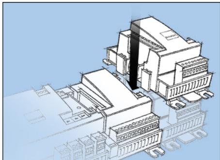
In our example two extension modules are to be fitted to the basic module. We have chosen to fit the module with relays directly on the basic module and then the module with input signals. The sequence is thus:
