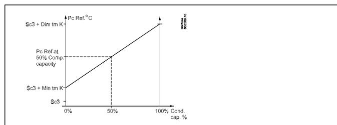
The minimum temperature difference (min tm) at low load should be set at approximately 6 K as this will eliminate the risk that all fans will be running when no compressors are running. Set the dimensioned difference (dim tm) at max. load (e.g. 15 K).
