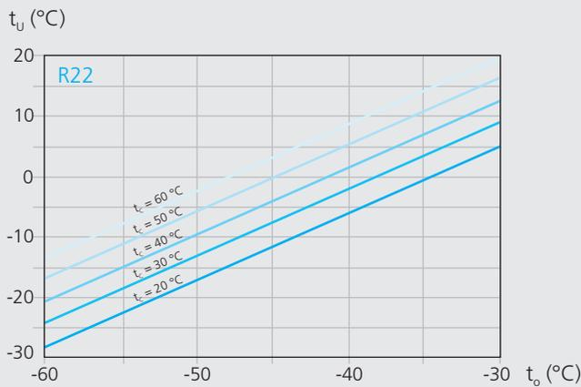
$t_u$  = Subcooling temperature at the intermediate cooler outlet (FUA)
