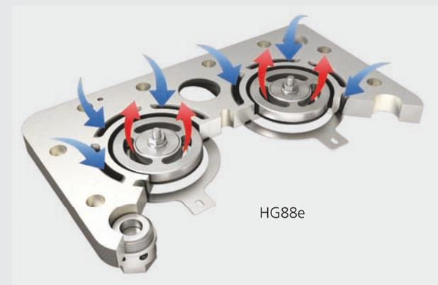
With the mexxFlow® system pressure losses can be minimized thanks to a flow-optimized double ring fin construction of the valve plate in combination with a cylinder head, which is specially adapted to the valve plate. Thus, the efficiency of the compressor can be increased considerably.
