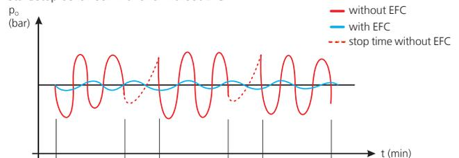
Capacity control in rack operation (4 compressors / of which 1 compressor with EFC)
