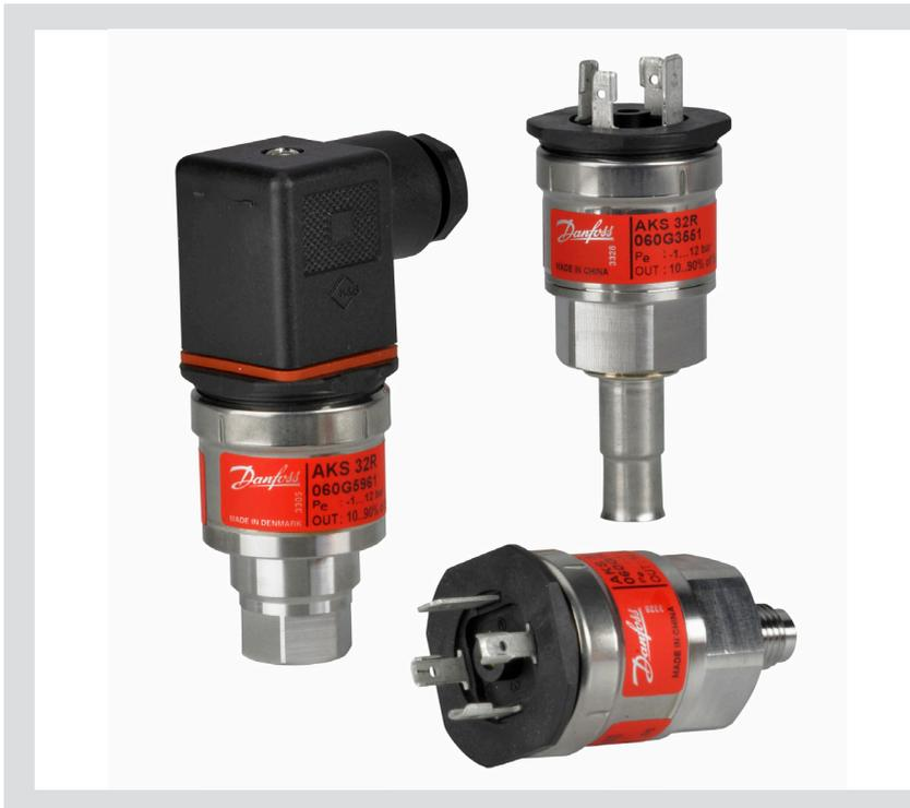
AKS 32R is a ratiometric pressure transmitter that converts the measured pressure to a linear output signal. The min. value of the output signal is less than 10% of the actual supply voltage. The max. value is more than 90% of the actual supply voltage.
