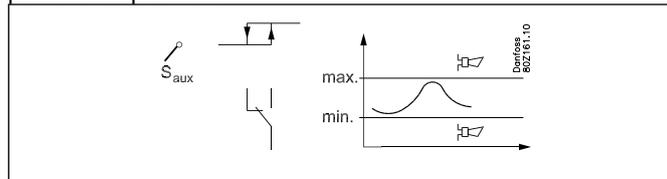
The thermostat can be used as one of the sensors S1, S2, S3, .. etc. Cutin and cutout limits are set for the thermostat. Coupling of the thermostat's output will be based on the actual sensor temperature. Alarm limits can be set for low and high temperature, respectively, including separate alarm delays. The individual thermostat function can be adapted to the relevant application as it is possible to give the thermostat a name and to indicate alarm texts.
