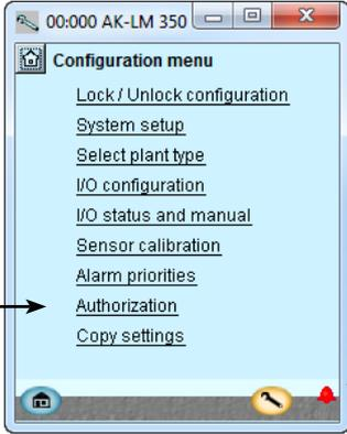
When the controller is supplied it has been set to show the default authorization for the different user interfaces. This setting should be changed and adapted to the plant. The changes can be made now or later.
