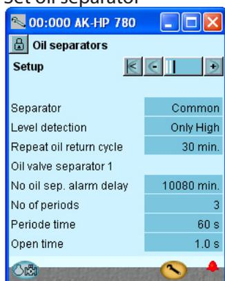
In our example, the oil supply is controlled separately for each individual compressor. The settings are shown here in the diagram. The process is as follows: 20 seconds after the signal from the level switch is given, the oil injection starts. This pulsates three times with one minute intervals. Each pulse lasts one second. Then there is a pause for 20 seconds. If the level switch has not registered any oil at this point, the compressor is stopped.
