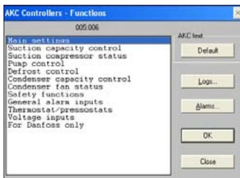
The operation is divided up into several function groups. When a selection has been made, push "OK", and you may continue to the next display. By way of example, "A Compressor capacity control" has been selected here.
