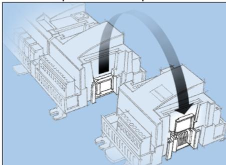
Remove the protective cap from the connection plug on the right-hand side of the basic module.
