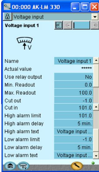
! When this function is set to 'YES', a relay will be reserved which couples with the voltage signal. Definition of the connection point must be done during the I/O configuration.
