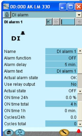
! When this function is set to 'YES', a relay will be reserved which couples with the digital input signal. Definition of the connection point must be done during the I/O configuration.
