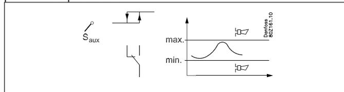
The thermostat can be used as one of the sensors Saux1, Saux2, Saux3, .. etc.
