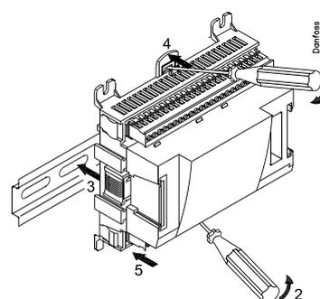
When the two snap catches for the DIN rail mounting are in the open position, the module can be pushed into place on the DIN rail – regardless of where the module is on the row.
