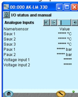
Before the control is started we check that all inputs and outputs have been connected as expected.
