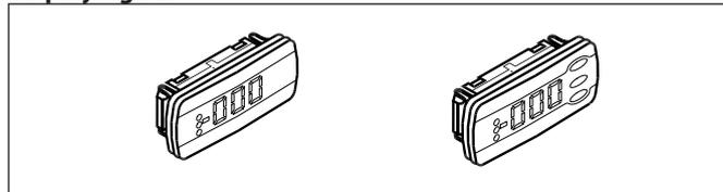
The values measured can be read from a display. This display must be of display type EKA 163B or EKA 164B. Up to four displays per controller can be fitted.
