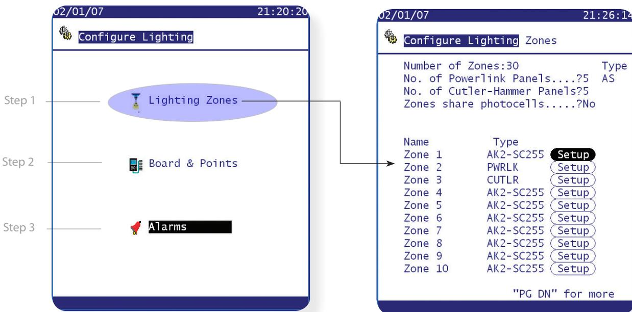
The Configure Lighting zone screen consists of the following areas - complete these areas to start the lighting configuration.
