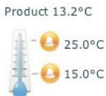
The 'Device Detail' page shows key data from the controller device. The simple thermometer icon indicates the upper & lower temperature alarm limits associated with the product temperature, with the actual 'product temperature' being shown above. Depending on controller device this temperature can be an actual sensor or can be a calculated via the controller. Consult the controller manual for further details.
