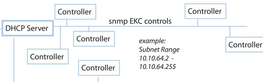
Check the box marked 'Channel SNMP'. SNMP is the protocol used to communicate with the EKC snmp controllers. Enter an address range for the AK-SC255 to scan in order to detect the EKC devices. For example, settings as IP address range (10.10.64.2 - 10.10.64.255).
