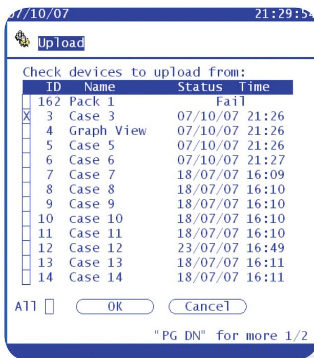
Access the upload function via the Refrigeration / Configuration / Controller Setup. Once in the controller Setup, the Upload button will be available. The resulting upload page will then make available all the controllers that have been scanned & configured in the AK-SC255.
