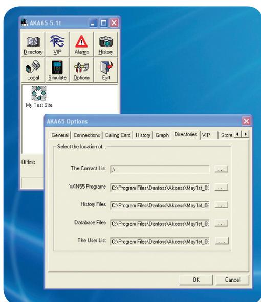
The WIN55 file is represented as a icon and is the program that the AKA65 uses to run the AK-SC255 environment. Ensure that the AKA 65 directories points to the folder that holds this file. The 'E' version of the AK-SC255 is denoted by the file name 'VExx\_xxx.exe'
