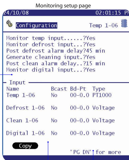
Page Down to access the alarm configuration for any defined inputs
