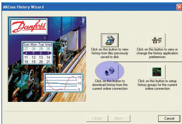
For this example, select and click the button that collects the history data via an on-line connection. This pre-pairs the process of pulling back the stored history data in the AK-SC255. The following screens will ask for data point selections and time retrieval periods.
