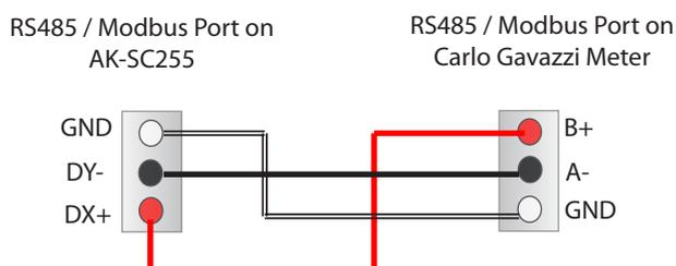
Once all communication wiring has been set, perform a network scan via the I/O network menu (ensure Modbus channel is checked in the Rescan page), the meter should be shown in the scanned list under the generic button.
