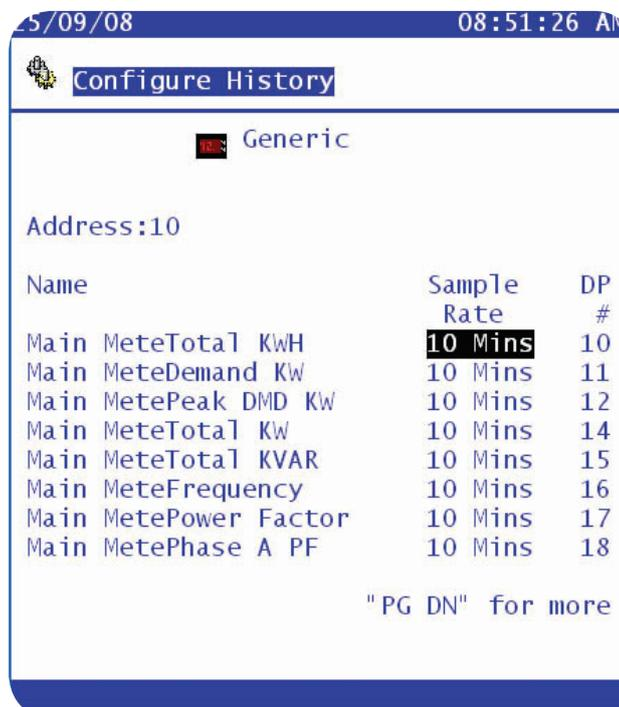
With a correctly fitted meter more detail of energy consumption is possible, the screens below give an example of this extended information.
