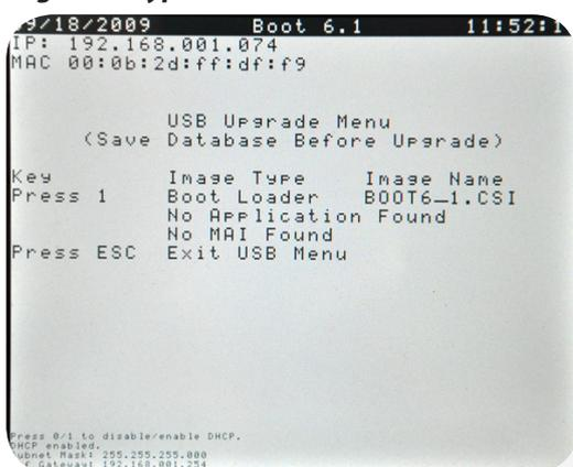
**Figure 6 - typical USB menu in normal run mode**
