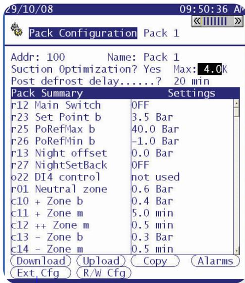
Once the level of offline controllers has been reached and the delay time has elapsed, the AK-SC255 will issue an alarm (based on the alarms settings), warning of optimization error - this alarm will be relative to the pack that is under this condition
