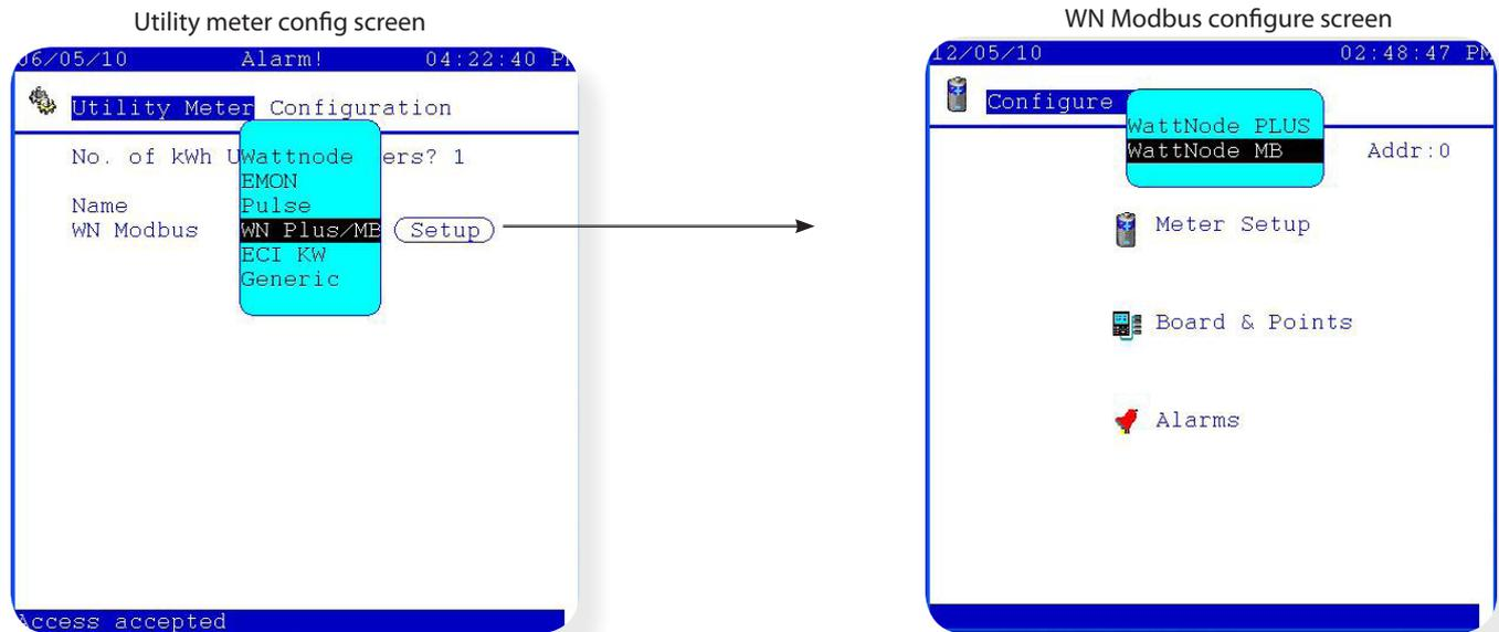
Enter the 'Meter Setup' screen, and the following areas are available for configuration;
