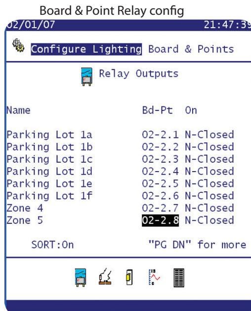
Dependent on how the previous Lighting Zone setup pages have been configured the Board & Point screen will reflect these settings. In the above example the initial **Relay page** shows 6 'Parking Lot' Zones - as per configured in the Lighting Zone setup. The Board & Point Input / Outputs that control these zones now need to be programmed.
