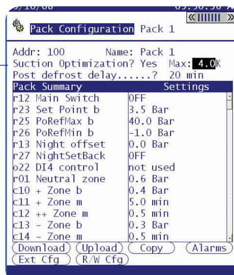
Use the pack controller 'Extended Configuration' to set optimization safety levels. Define the number of controllers offline that will stop Po Optimization (and subsequently issue an alarm). Define a time delay before Po Optimization is de-activated. Define an alarm action.
