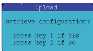
A prompt to retrieve data from the controller may show – by selecting 1 (yes) the AK-SC255 will retrieve all the current values and settings in the drive so that the AK-SC255 database and screen are synchronized with the current drive settings.
