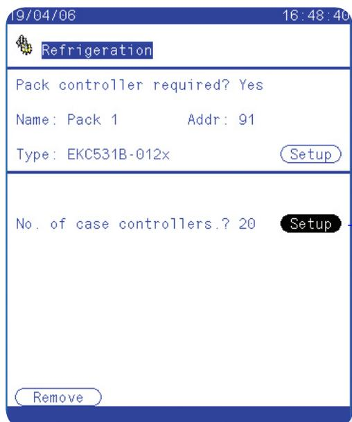
A number of evaporator controllers will now be displayed. At this page select the controller type via the drop down list.
