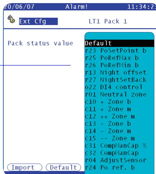
Only temperature or pressure parameters will function with the status value change function.
