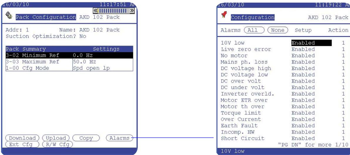
Once all configuration of the drives has been completed the resulting details can now be seen from the main menu. Depending on how the drive was configured (as 'pack controller' or 'stand alone') the drive details will be seen under the Drive or Pack icons.
