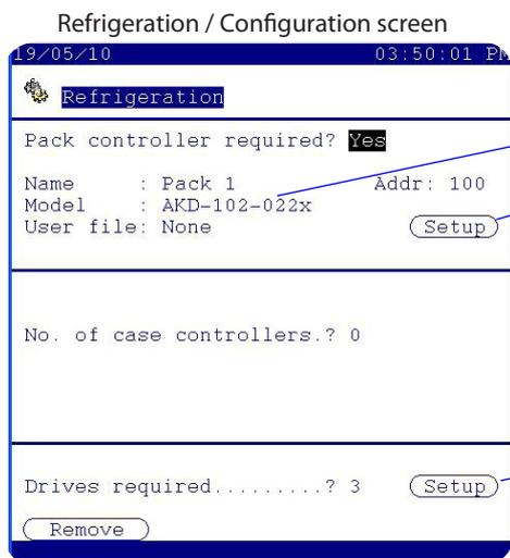
If the AKD 102 is to be used as a **pack controller**, configure AKD-102 type and use the Setup button to access drive parameters
