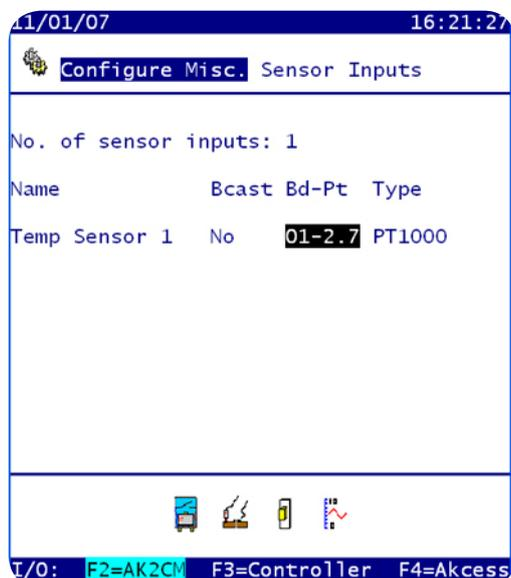
In this example, when programming the AK-SC255 simply type 0127 and the format will be automatically set for AK2 I/O.
