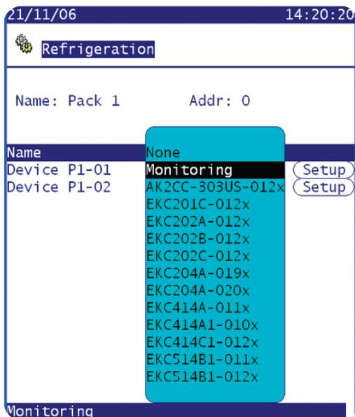
To setup monitoring points follow the 'standard' method in refrigeration configuration - Main Menu / Configuration / Refrigeration / Add Controls. Answer 'No' to the question 'Pack controller required?' and navigate to the lower section of the screen and describe how many monitoring sensor points are required (still described as No of case controllers.?)
