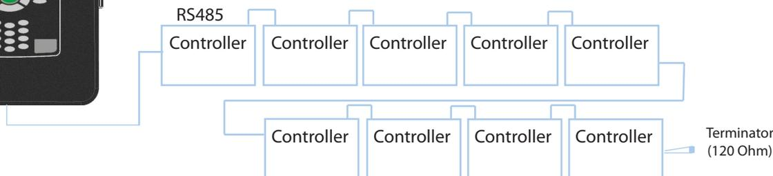
Once the network is complete, select Lonworks® check box and the AK-SC255 will automatically scan for all addressed devices on the network. (**Address range 1-199**).
