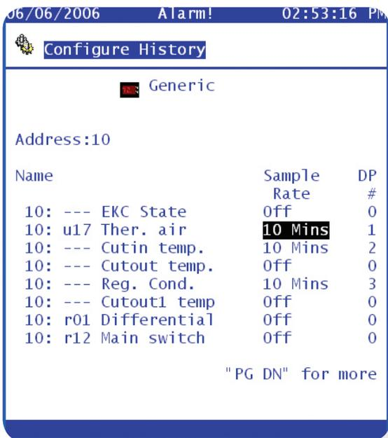
To make a change in any one of the controllers listed, highlight the device and press enter.
