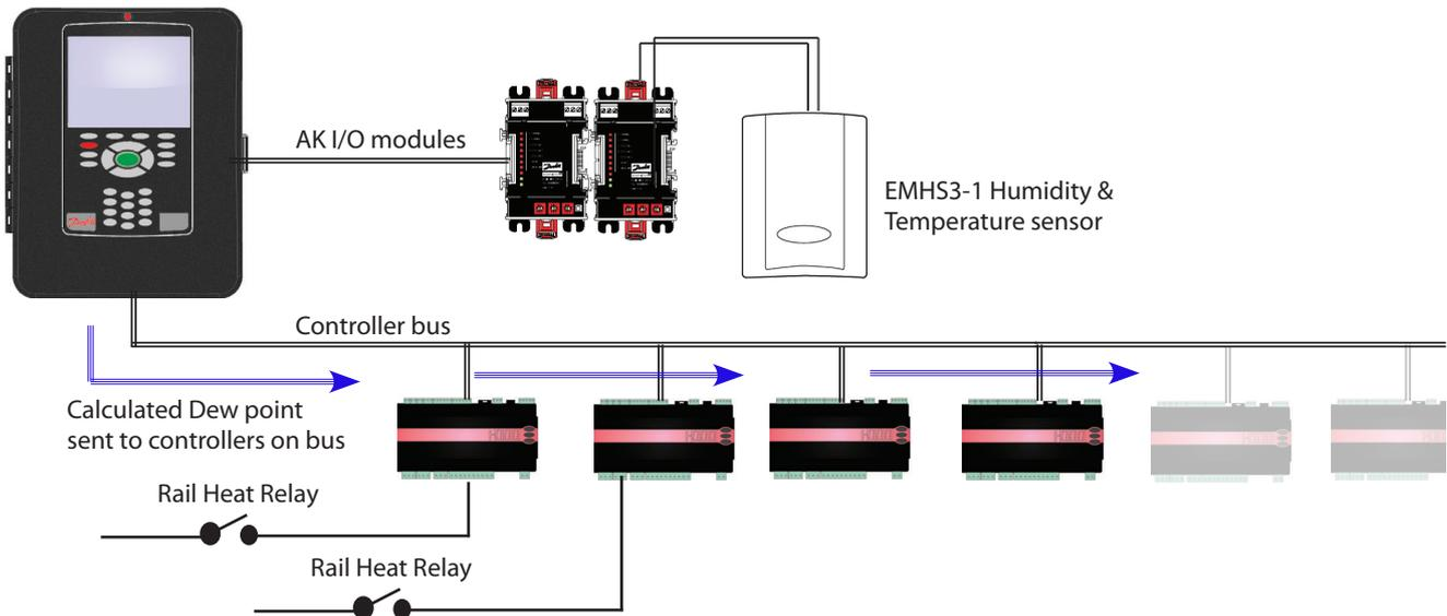
Before configuring rail heat in the AK-SC255, the AK-CC 550 controllers require setting. Review parameters o85, o86 and o87, as noted below.
