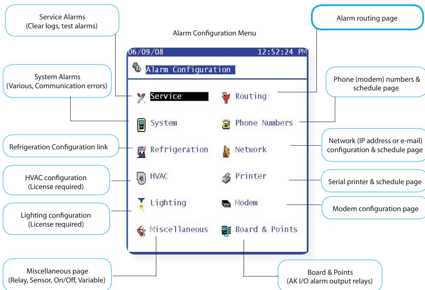
2/ When in the alarm routing page, an array of output routes (including relays (A-J), Modem, e-mail, will be presented along with the Alarm Actions (1-8) and the associated action stop conditions.
