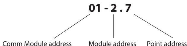
No matter what the address is set on the communication module, the first connected AK2 module will assume the address 1.
