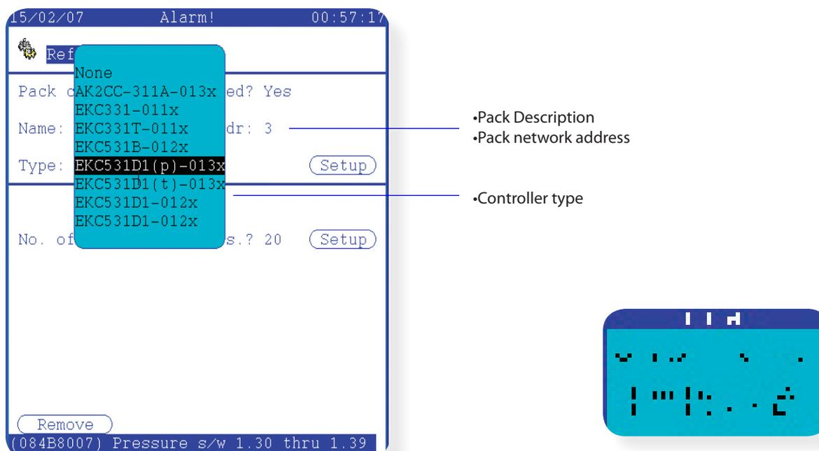
Next select the setup button and a pop up dialog box will appear to ask if the controllers configuration is required to be uploaded. If the Pack controller is powered up, correctly addressed and is present on the network option 1 can be made.
