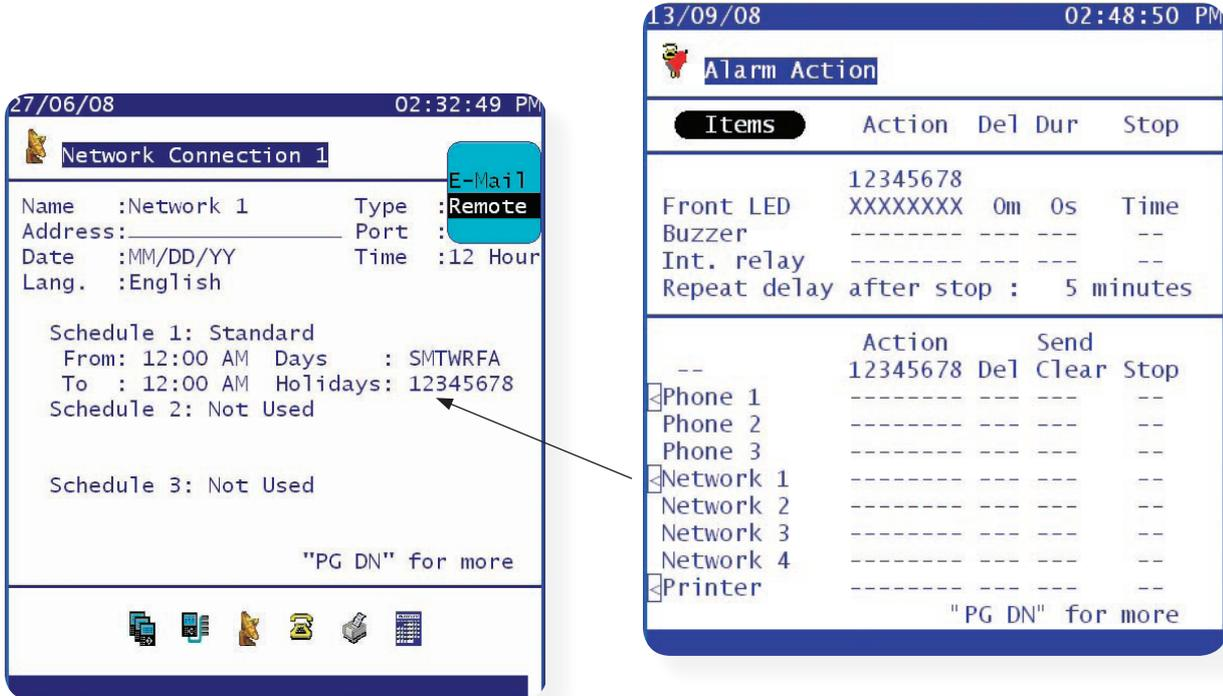
The final screen in the Alarm routing setup provides the option to identify which AK-SC255 will be used to output the alarms. In applications where multiple AK-SC255 units are interconnected, use this page to define which AK-SC255 issues out the alarm outputs.
