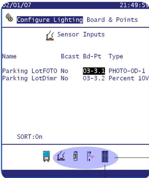
Check & configure the remaining Input / Output areas of the Board & Point lighting
