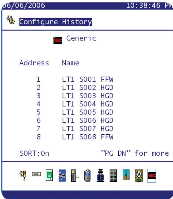
Having selected 'Generic' the available connected controllers will be displayed. The list will indicate the controllers net ID address and the description.
