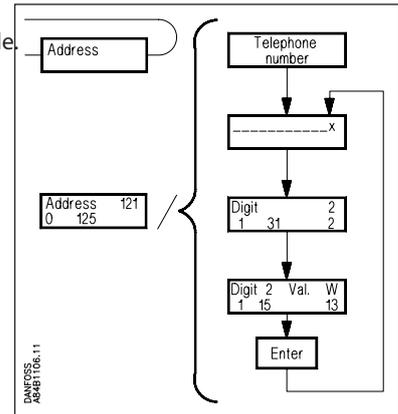
The actual telephone number for the selected line in the router table. The telephone number may consist of up to max. 30 significant digits composed of figures and modem codes. All telephone numbers must be terminated with 'x' (see below).
