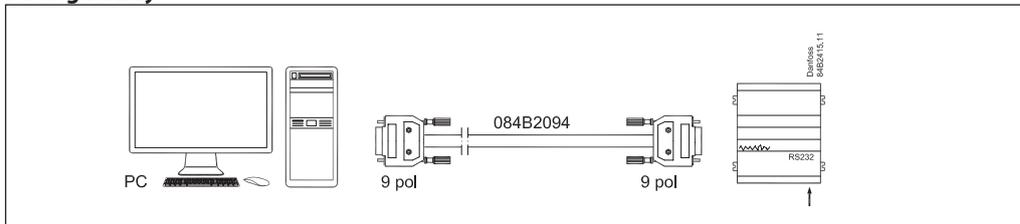
A 3 m cable with plugs fitted can be supplied. See Ordering.
