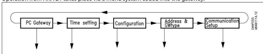
The gateway menu structure has been “lowered” in relation to the menu structure of the AKC controllers. Change between menus takes place by means of the control module’s arrow keys.
