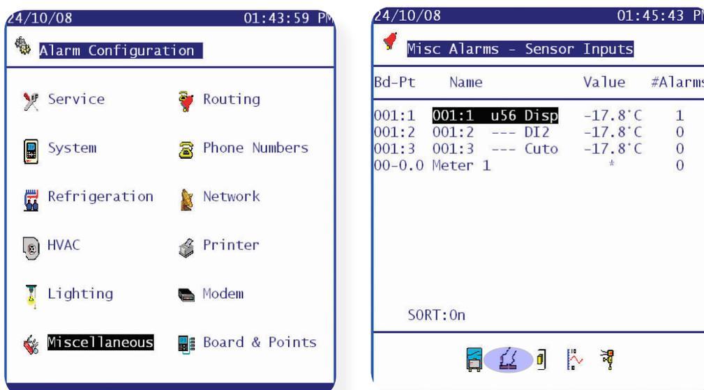
When in the alarm configuration page for the import parameter select the number of alarms required (max 3). Complete the alarm configuration by setting the alarm action and alarm limits, including the alarm action number.
