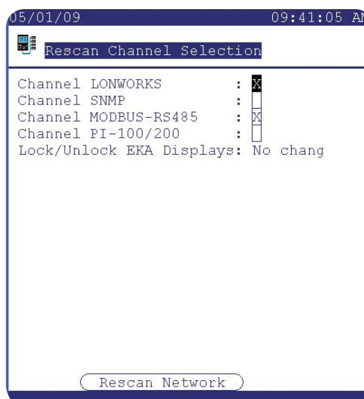
Rescan Channels page showing the Modbus and Lonworks ports selected. Press the Rescan Network button to scan network
