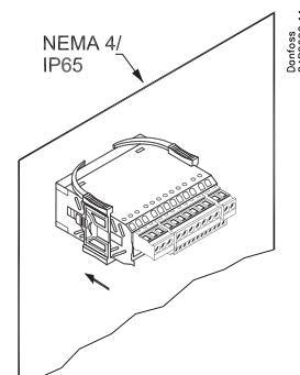
$t_{amb} = 0 - +55^{\circ}\text{C}$ 084B8506 = 230 V a.c.
