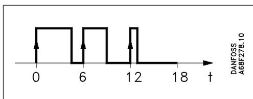
The relation between this opening and closing time indicates the actual capacity. If there is an intense need for refrigeration, the valve will remain open for almost all six seconds of the period. If the required amount of refrigeration is modest, the valve will only stay open during a fraction of the period. The amount of refrigeration needed is determined by the controller.
