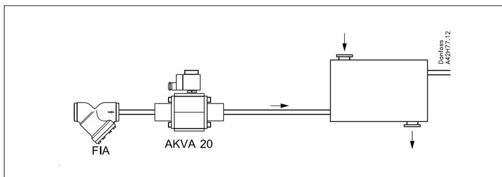
**Electrically operated expansion valves, type AKVA 10, 15 & 20**
