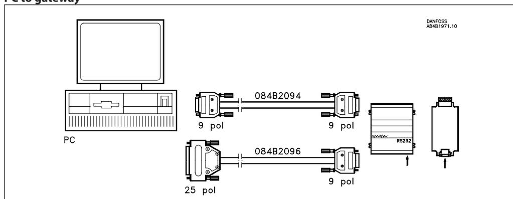
Check whether the PC has a 9-pole or a 25-pole plug for this connection. A 3 m cable with plugs fitted can be supplied. See Ordering. If the cable has to be longer than 3 m, mount it based on the following instructions:
