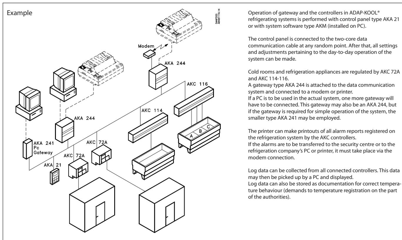
The same functions can be carried out with gateway type AKA 243, but here it is also possible to communicate with other controllers via the LonWorks output. The output will primarily be connected to controllers from the EKC 200, 300, 400, 500 or AK 2 series.
