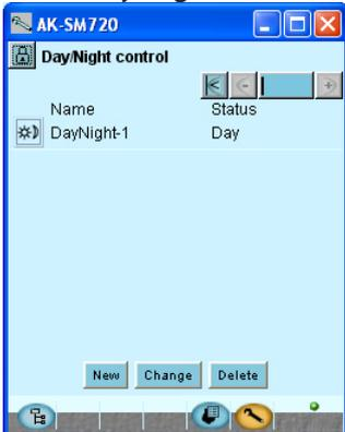
Groups established via this operation receive the day/night signal at the same time. Activation of the signal either takes place from a schedule and/or from a switch.
