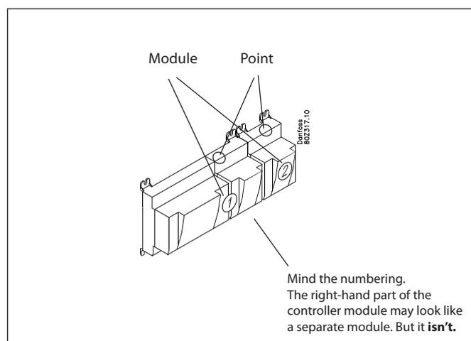
The connection survey from the controller and any extension modules are uploaded from the paragraph "Modules". See later in the manual E.g. controller module:
