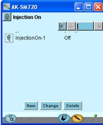
Groups established via this operation receive a signal so that liquid injection is stopped. Activation of the signal takes place via a compressor control.
