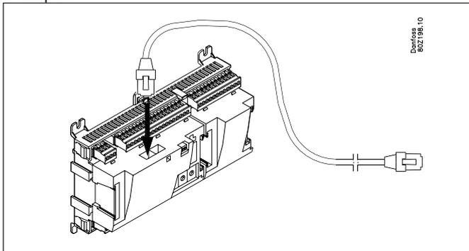
A HUB, Switch or Router can be connected as required. If a HUB or Switch is used, the system manager must be assigned a fixed IP address.
