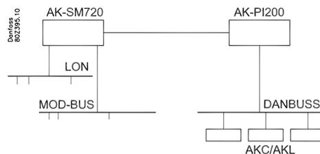
This function is only used if the system manager needs to exchange data with controllers of the type AKC which are controllers with DAN-BUSS data communication.
