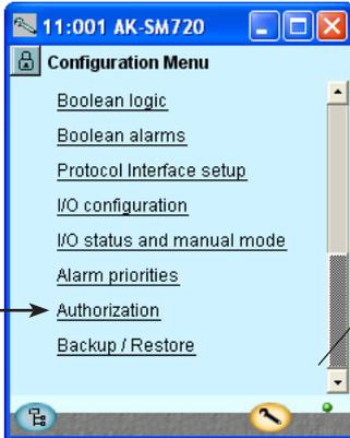
When the controller is supplied it has been set with a standard authorization for different user interfaces. This setting should be changed so it is adapted to the plant. You can change this now or later.
