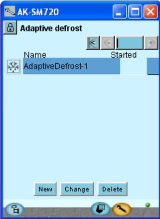
A group created via this control will use the "Adaptive defrost" function. The controllers in the group receive signals of the current condensation temperature from the condenser control. Only controllers with this function can be selected for the group.
