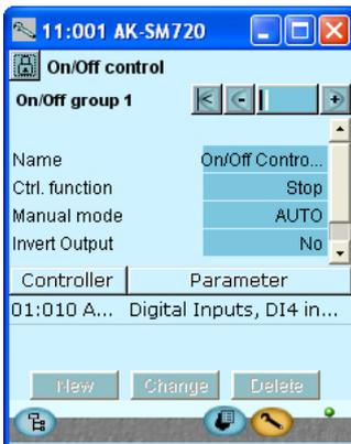
The groups that are set up via this control can collect signals from one On/Off function in any controller on the network. This signal is then forwarded to another On/Off function on the network.
