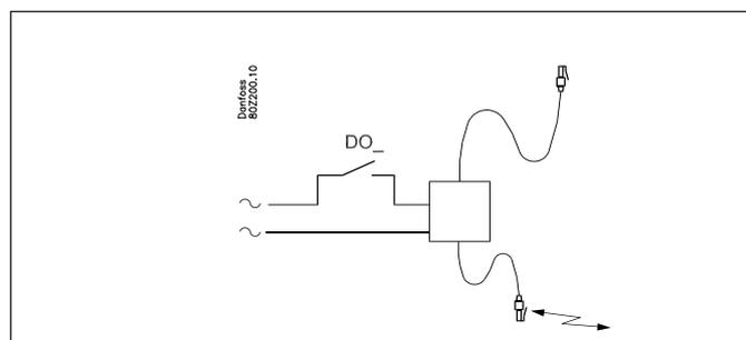
The supply voltage to the modem must be connected via a relay output. This enables the system manager to reset the modem. The modem will also be switched on and started in a controlled way when the system manager is switched on.
