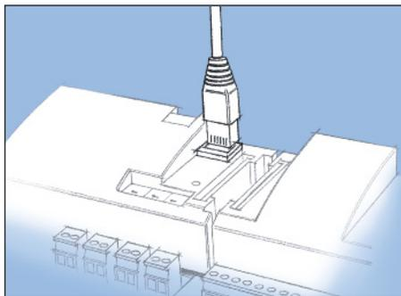
The plug from the Service tool programme is removed from the controller and the modem plug is connected in its stead.
