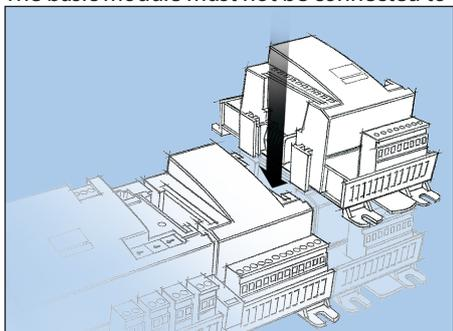
In our example one extension module is to be fitted to the basic module.
