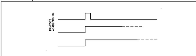
To provide security, a time must be set in the individual controllers. There is a maximum permitted hold time to wait for the start signal for refrigeration. If this time is passed, refrigeration will be restarted regardless of signals from data communication.
