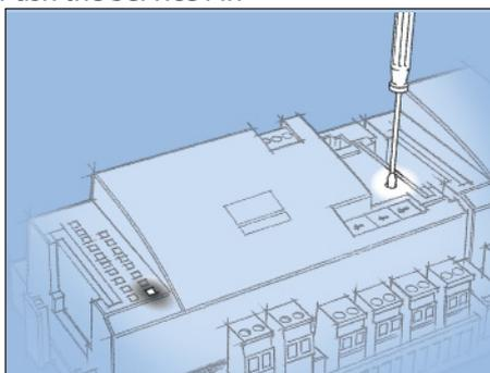
Press down the service pin and keep it down until the Service Pin LED lights up.
