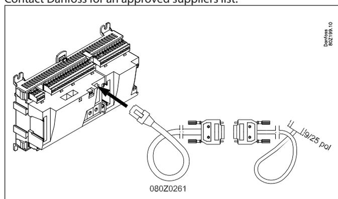
The modem is connected to the socket on the front (the same socket that a Service tool uses).
