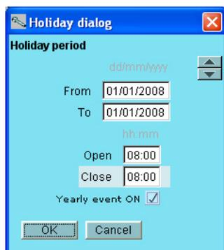
A schedule must be established that indicates the shop's opening hours. The schedule is later to be used in connection with day/night operation of refrigeration appliances. (The day/night changeover can be set relative to this schedule. A later change of opening hours will merely require an adjustment in this schedule.)
