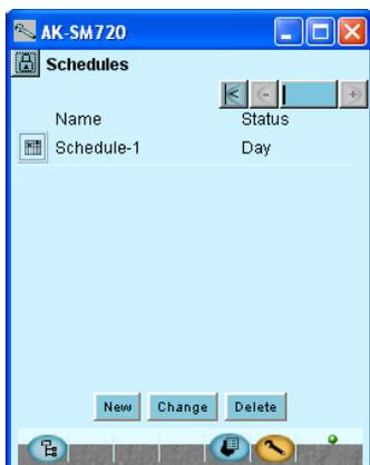
Schedules set up via this operation can be used for day/night signal. The signal is transmitted via the data communication to selected controllers.
