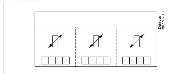
Up to three groups of evaporator controls can be defined. Each group must have its specific dew point sensor. The dew point sensor must be located in the same room as the refrigeration appliances that are to receive the signal.
