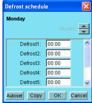
If there are several days with identical defrost processes, use the copy function. The end result with two defrost processes a day can be seen in this screen.
