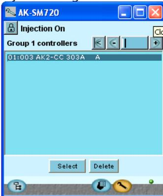
The picture to the left shows the final result. The controllers have been selected via the "Select" button. Only select controllers belonging to the selected suction group.
