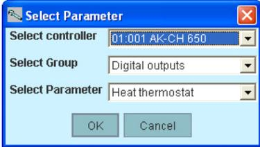
When the OK button has been pressed, the function receiver can be seen in the previous display.
