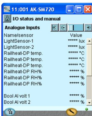
Before the system manager is started we check that all inputs and outputs have been connected as expected.
