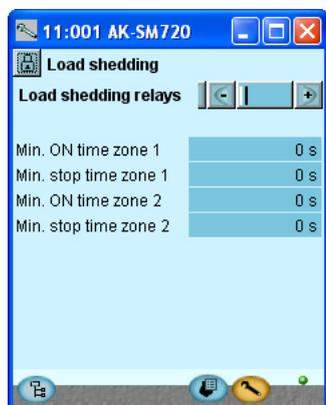
This function can only be used together with the earlier "Consumption measurement" function. If consumption rises to a peak situation, some of the load can be disengaged so that consumption does not exceed a defined value.
