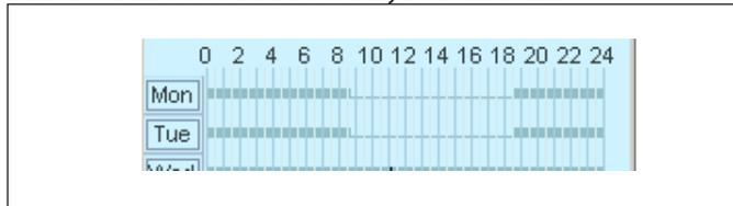
Both types of schedule can be overridden with a switch function. If the switch is activated when the schedule is off (night), it will create an on (day) status.
