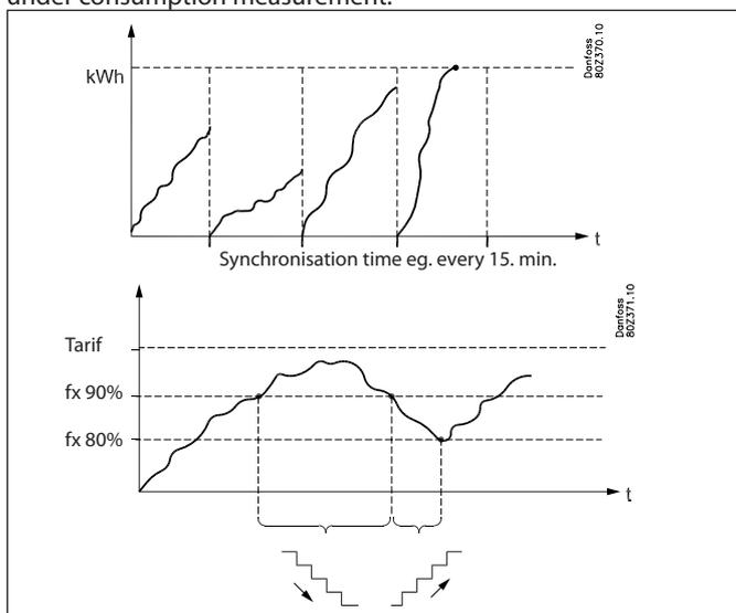
At the beginning of a period all consumption will be engaged during an adjustable period of time, so that the function has a basis for calculation before control commences.
