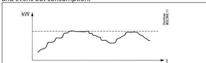
Consumption is monitored within a measurement period. If consumption rises above a limit, consumption will gradually be disengaged with the aid of relays. Once consumption has fallen below the limit once more, re-engagement takes place. Disengagement can take place in ten steps.
