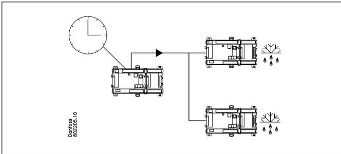
The defrost process start can come from a weekly schedule or from a switch function connected to the system manager. When defrost has started, it is up to the individual controllers to determine how it is concluded. Some based on time, others based on temperature.
