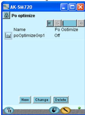
Groups established via this control will follow the temperature in the selected cooling sections and transmit a signal to the compressor control to the effect that the suction pressure can be displaced.
