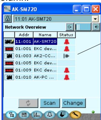
There is now access to all the connected controllers. If they have not already been set up individually it can be done via data communication from the system manager, or the modem may be cut in and the setup can then take place via the modem communication.
