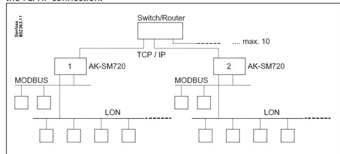
Controllers with DANBUSS data communication can be connected via a TCP/IP connection. The same applies to wireless units
