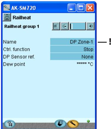
! If you enable this function, two lines will automatically be created and reserved in the I/O configuration. The lines will contain the name of the function. In these lines you must set a Module Number and a Point Number. See also page 60 onwards.
