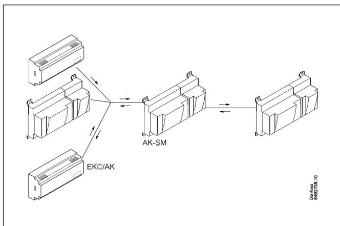
The main function of the system manager is to transmit alarms. It also contains the primary functions that the refrigeration system's controllers can use to sub-optimize the individual refrigeration sites.
