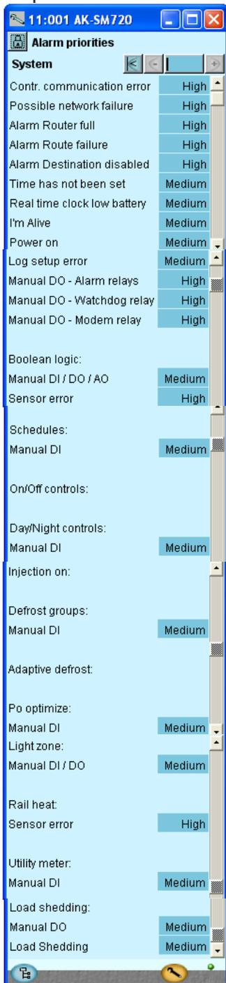
Very many functions have an alarm connected. Your choice of functions and settings has connected all the relevant alarms that are current. They will be shown with text in the three pictures.
