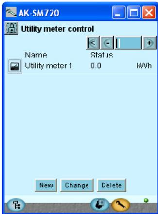
This function will require a signal from a pulse counter. Consumption can then be monitored in the screens displayed. Up to eight measurements can be set up.
