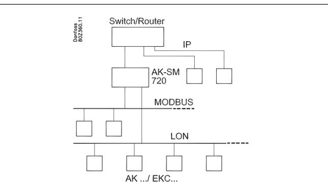
All controllers on the data communication must have an address set before this point is carried out.
