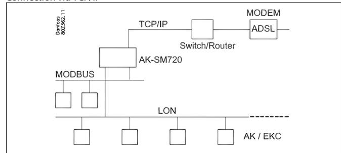
In larger networks several System Managers are connected to one another via the TCP/IP connection.
